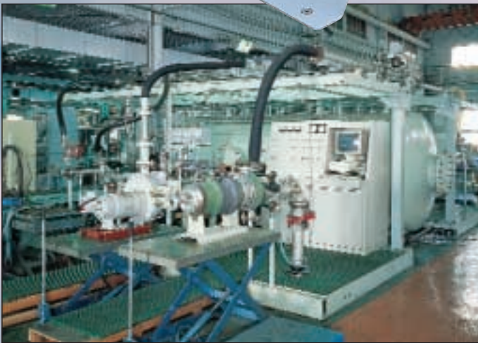
In Teikoku's factory testing lab, all pumps are 100% performance-tested before shipment.
